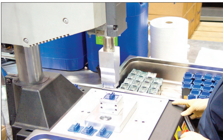
MSE's Patented Welding Technologies are also used in the company's inkjet facility.
