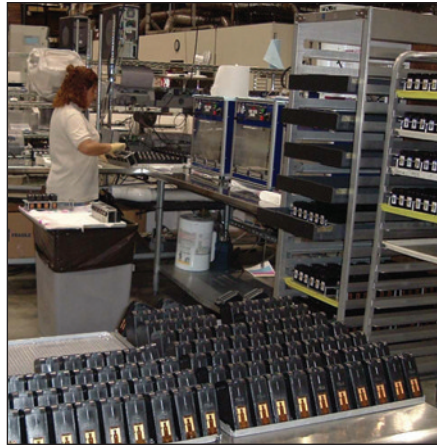
Left: MSE has expanded its inkjet offerings and now manufactures more than 12 print-head-based models. Inkjet capacity exceeds 150,000 inkjets per month. Right: MSE engineers also design and manufacture equipment such as the HP 56 inkjet filling station in-house.
